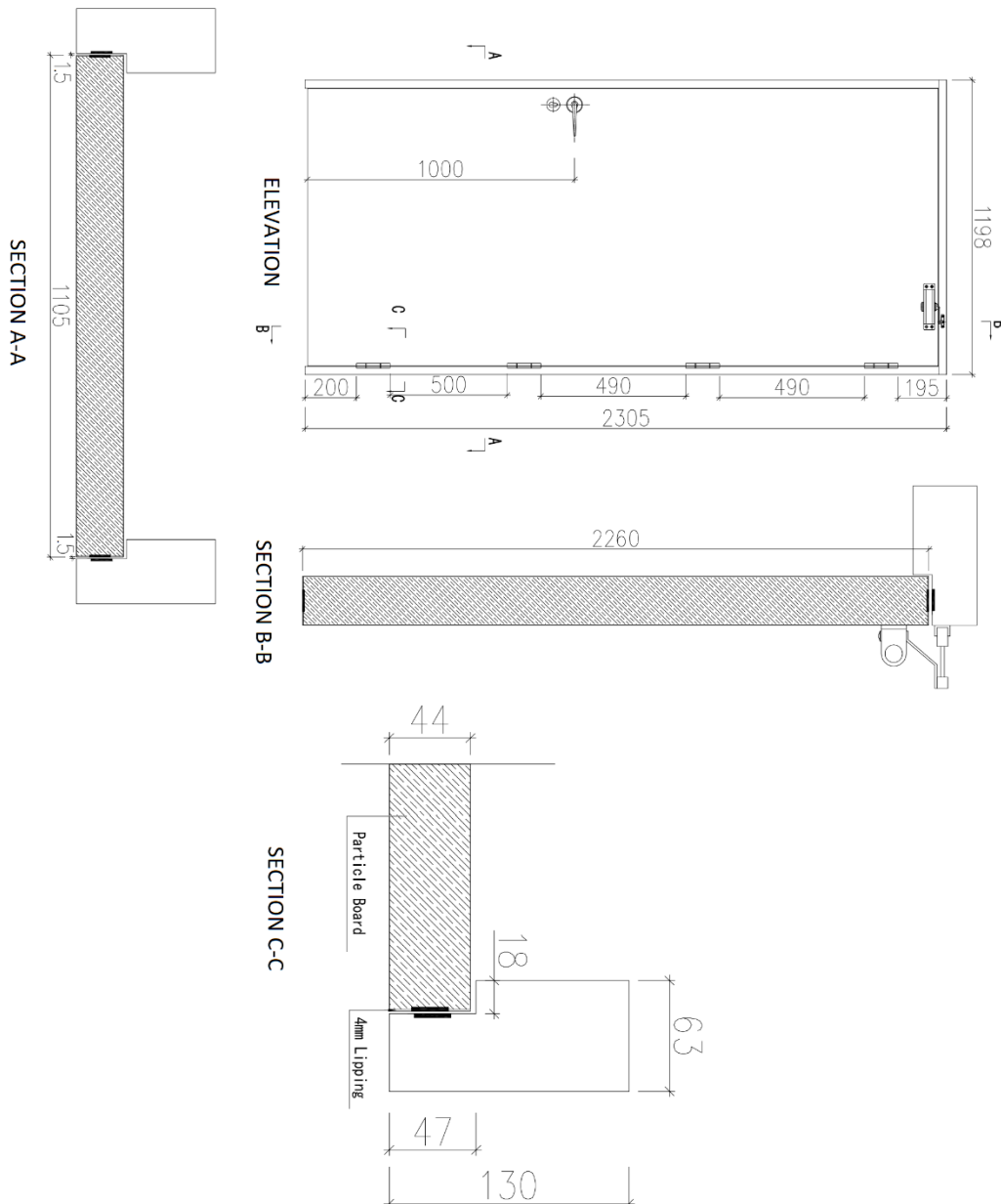
Assembly Drawing of single leaf timber door with particle board core, model of MS-001A
