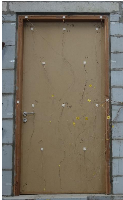
Fig. 2 Unexposed Side Prior to the Fire Test
