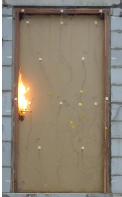
Fig. 7 Unexposed Side after 36 Minutes
