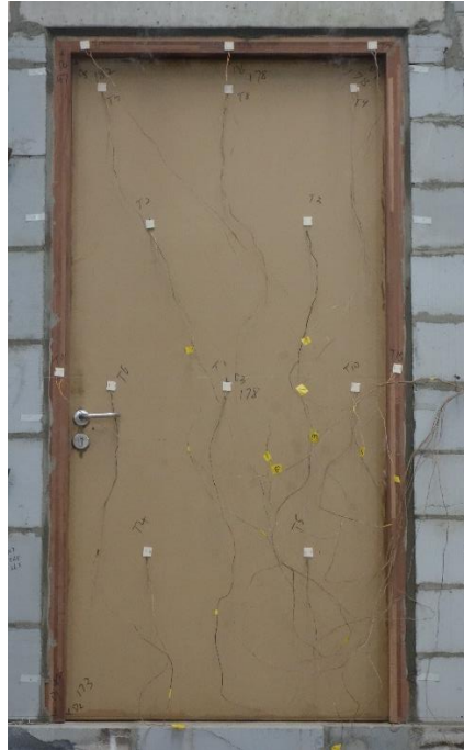
Fig. 3 Unexposed Side after 10 Minutes
