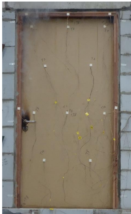
Fig. 6 Unexposed Side after 34 Minutes
