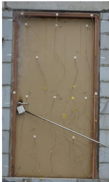
Fig. 4 Unexposed Side after 28 Minutes
