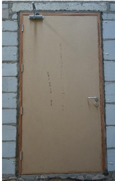
Fig. 1 Exposed Side Prior to the Fire Test
