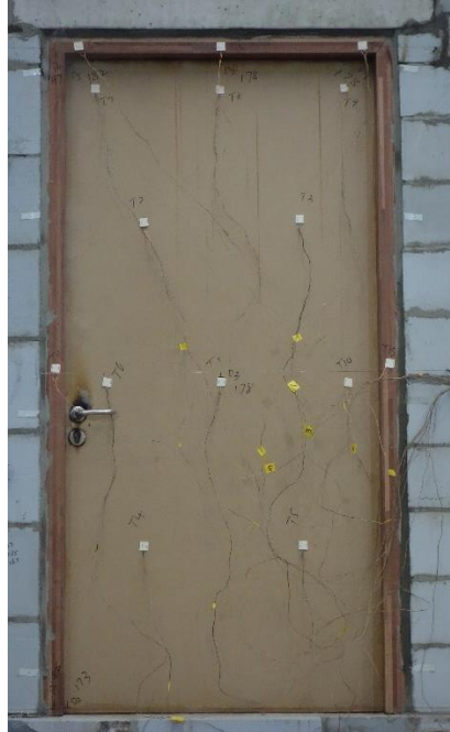
Fig. 5 Unexposed Side after 30 Minutes
