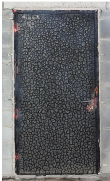
Fig. 8 Exposed Side after 36 Minutes
